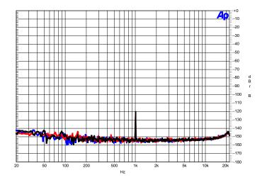
The conventional test for dynamic range requires a -60dB output. In testing the M2, we have gone several steps further in also testing with -120dB. It is remarkable that this small signal level is resolvable. It is also notable that the performance remains exactly the same over a broad range of volume settings. The chart shows identical performance over three gain settings separated by 40dB.
