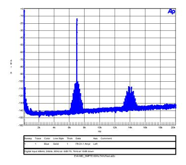
SMPTE Intermodulation spectrum is very clean with all distortion products below -100dB or 0.001%.
