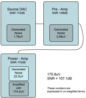
This 107.1dB figure is referenced to a 200W output power. Stating it referenced to 1W, gives a figure of 84.1dB. This is the true end-to-end performance of even this exceptional conventional signal chain. Even the outstanding power amplifier used in this example cannot help, if noise is presented at its input.
