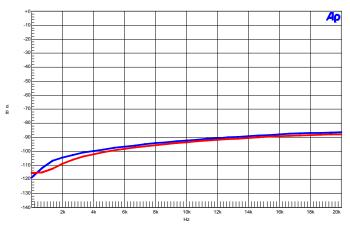
Channel Separation is greater than 90dB all the way up to 10kHz and still 85dB at 20kHz, which is 10dB better than the best analogue stereo integrated amplifiers.
