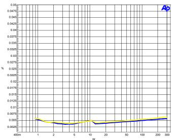
The familiar measurement of THD+N vs. output level shows the expected level of performance for a high-end amplifier. However, much more is revealed by looking at the M2 performance in terms of low level detail.
