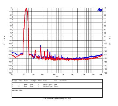
Distortion spectrum of 60Hz signal at 250 watts into 8 ohms shows a very clean spectrum with higher order harmonics well suppressed.
